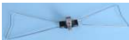
“Bow Tie” UHF antenna (300 to 800 MHz)
