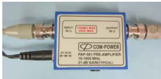
Com-Power preamplifier, gain 21 dB, 10 – 1000 MHz, $475 (Measured range was 3 MHz to 1.5 GHz+).
