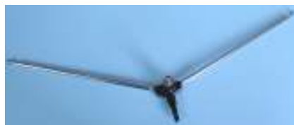
Adjustable “precision” dipole (65 to 200 MHz)
