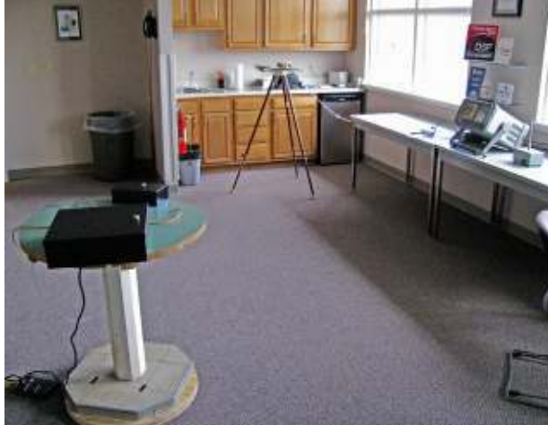
3m test range set up in a conference room.
