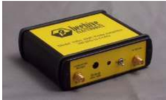
Beehive preamplifier, gain 30 dB, 4-5 dB NF, $525. Courtesy, Beehive Electronics.
